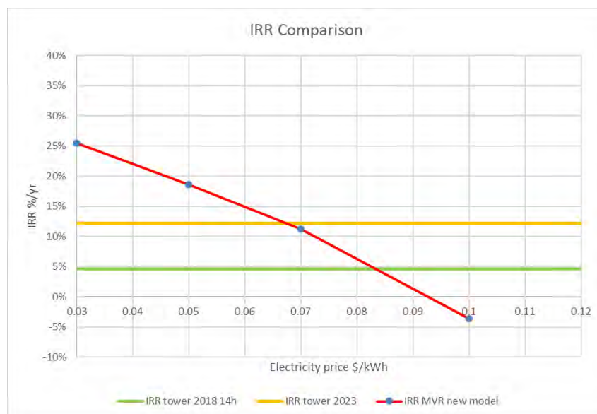
Figure 37: Comparison of IRR for solar thermal with MVR steam production (Assumptions: lifetime: 20 years, gas price: $10/GJ, boiler efficiency: 82%, CO 2 emissions cost ($29/t in 2020 to $131/t in 2050, O&M cost: 2% of capex per year).
