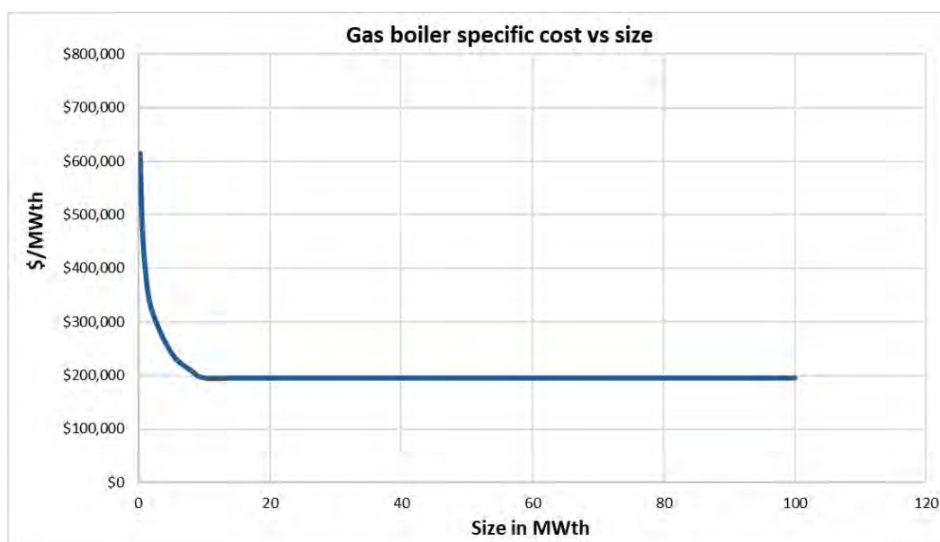
Figure 20: Gas boiler specific cost versus size.
